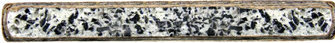
Cross-section of typical 1x6 Lead Edge Board Illustrates Exoskeleton and recycled rubber filled core
